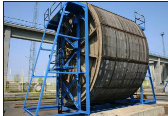
The drum screen prior to protection
