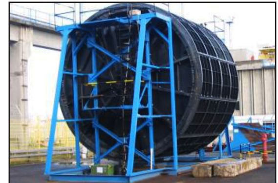
Completed application including ARC protection, and new shaft seals and bearing protection
